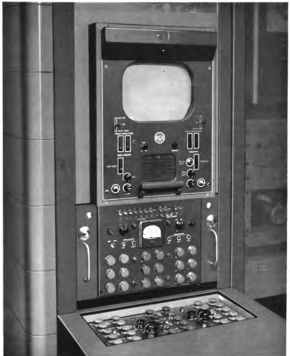
FIG. 28. Either the film or studio camera controls may be mounted in a standard rack shell as shown here. When this is done the monochrome monitor is usually mounted directly above the camera control position and the color monitor in the adjacent rack at about the same eye-level. An arrangement of this kind saves floor space and is convenient for setup and maintenance. It is particularly useful in installations where the camera control position is in a room separate from the studio control room.
