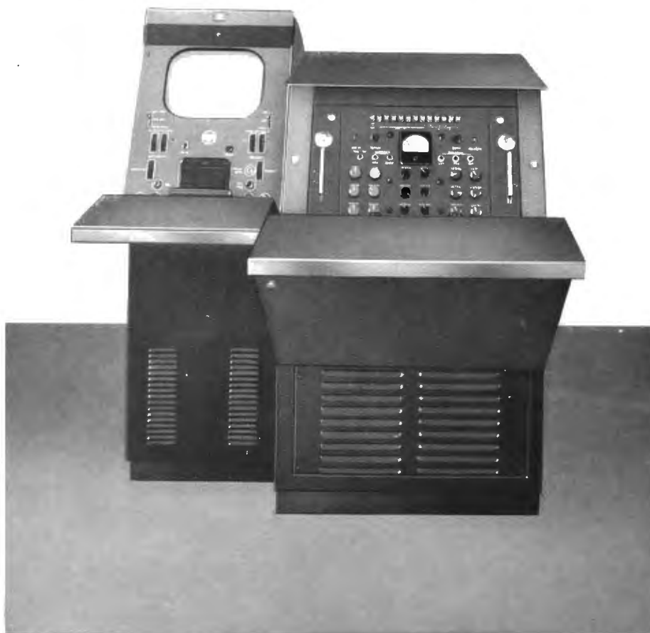
FIG. 27 (left). The studio color camera console includes a monochrome monitor (left) and a 19-inch console housing the processing amplifier and camera control panel. These units may be located at a separate position or assembled with the monochrome control consoles. The color monitor may be suspended from wall or ceiling (for easy viewing) or placed on the flat top of the 19-inch console (see Fig. 16, page 42). Alternatively both monochrome and color monitors, as well as camera controls, may be rack-mounted as shown in Fig. 28.
