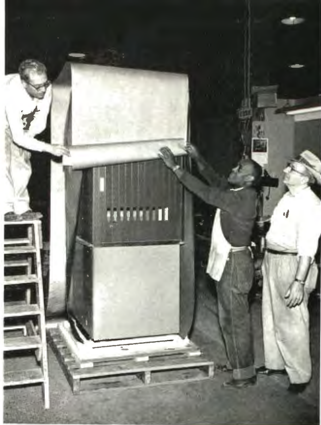
One of the cabinets (left) of the TTU-25A Amplifier is placed in temporary packing for its short trip to Wilkes-Barre. Right, another cabinet gets a final check before shipment. The amplifier equipment is comprised of six individual sliding door cabinets of this type.
