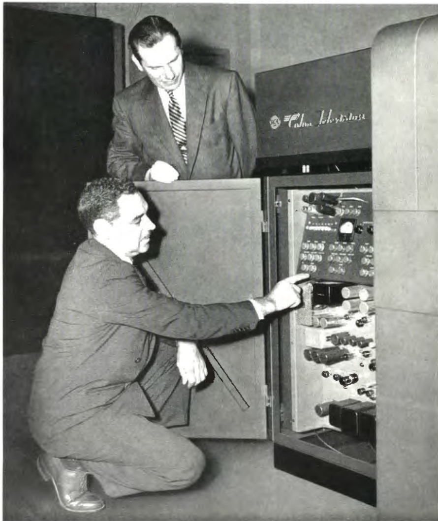
FIG. 18. A. R. Hopkins, Manager of RCA Broadcast Equipment Marketing and C. G. Nopper, Chief Engineer of WMAR-TV, Baltimore, are inspecting the control panel of the "3-V" Color Film Camera. This view of the 3-Vidicon Camera pedestal shows the location of vidicon enclosure atop pedestal, local control panel, and camera auxiliary panel.
