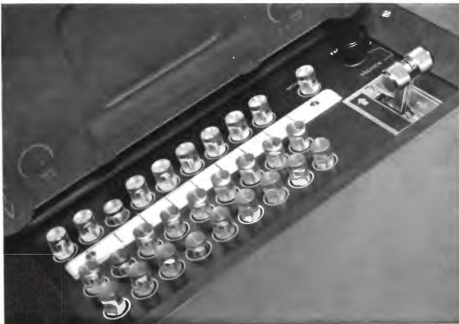
FIG. 1. Close-up of TS-11A Control Panel. The lower two rows of pushbuttons feed any of nine input signals to the faders. The upper row is for preview. A Program Transfer Switch (above the faders) allows Preview and Fader channels to be transposed for special program applications.
