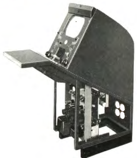
The TS-11A Switcher is supplied with an RCA console housing (MI-26266-B), a TM-6B master monitor and power supplies to form a complete versatile system.
